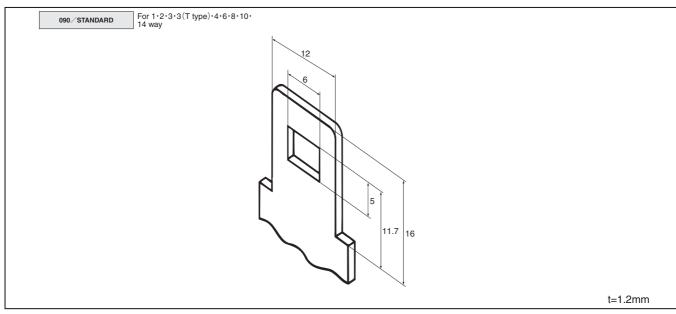
Note) The dimensions as shown here are reference dimensions and detail dimensions for mounting portion of the bracket are specified in the official drawing. Please contact our sales staff.
